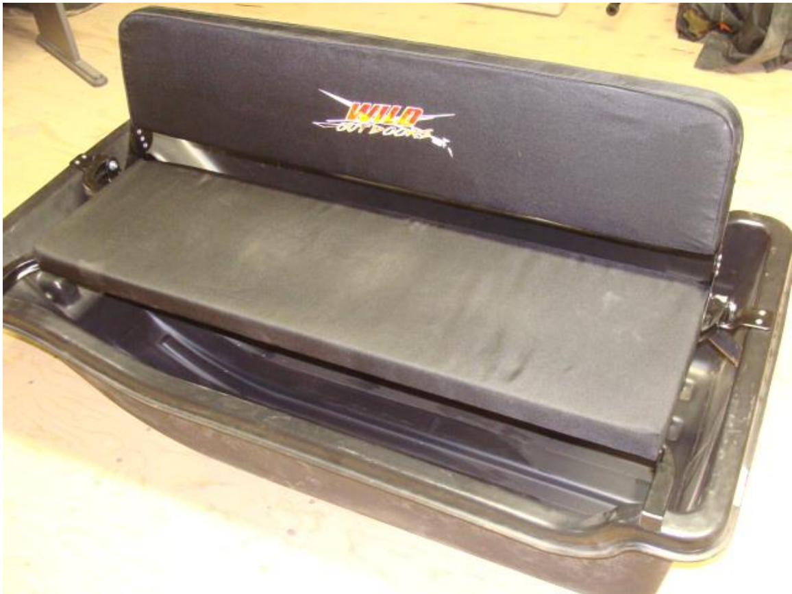
Completed bench is offset toward the rear of the sled to minimize tipping of the sled due to the front angle on the sled.
